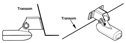
Position transducer mount on transom and mark mounting holes. Side view shown (left) and seen from above (right).
